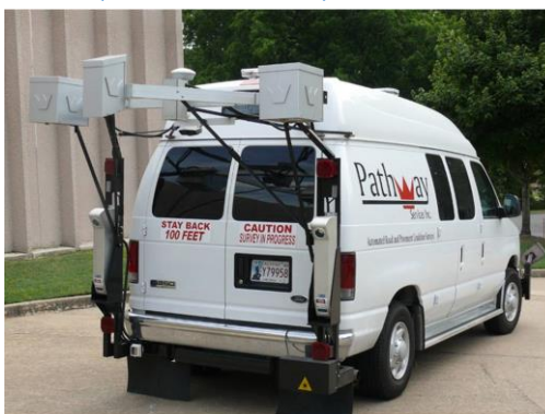
PathRunner collects pavement images www.pathwayservices.com/
