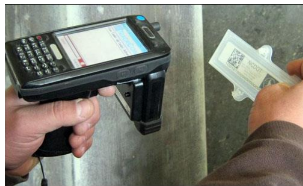
RFID Scanner and label prior to being attached to product.
