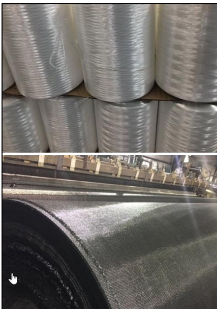
Spooled polypropylene yarns before manufacturing (top), geotextile product after weaving (bottom) – images from Foundation Geotextiles website
