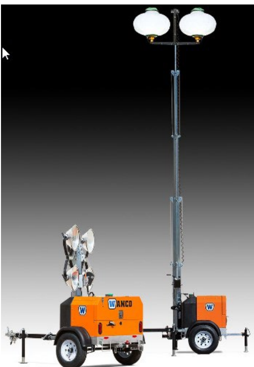
Image of the Wanco Diesel Tower with Dual Balloons at full extension along with a retracted view of Wanco’s Compact Light Tower with alternative light option from Wanco’s product brochure.
