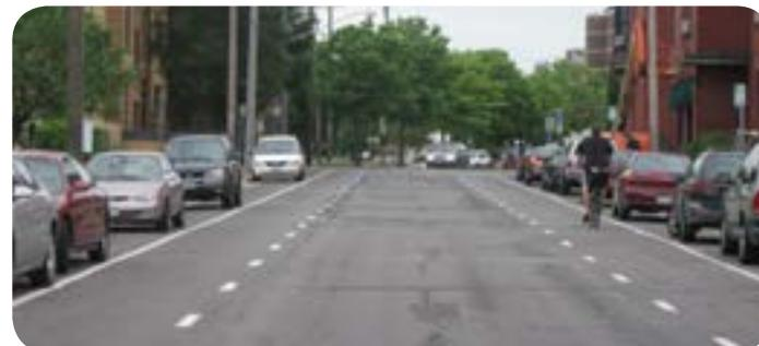
**Uphill Climbing Lane:** On streets where downhill grades are long enough to result in bicycle speeds similar to typical motor vehicle speeds, a bike lane may be provided only in the uphill direction with shared-lane markings in the downhill direction. This design can be advantageous on streets where fast downhill bicycle speeds have the potential to increase the likelihood of crashes with fixed objects, particularly in locations with on-street parking. (AASHTO)
