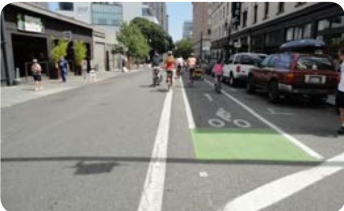
**Two-Way Cycle Track:** Two-way cycle tracks are physically separated cycle tracks that allow bicycle movement in both directions on one side of the road. Two-way cycle tracks share some of the same design characteristics as one-way tracks, but may require additional considerations at driveway and side-street crossings. (NACTO)
