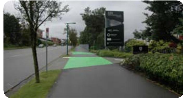
**Consolidated Driveways:** Driveway crossings of sidewalks often create hazards for pedestrians as motorists may not be looking for pedestrians as they pull into or out of a driveway. Where multiple driveways exist in close proximity, efforts should be made to consolidate the driveways and reduce conflict points with pedestrians.
