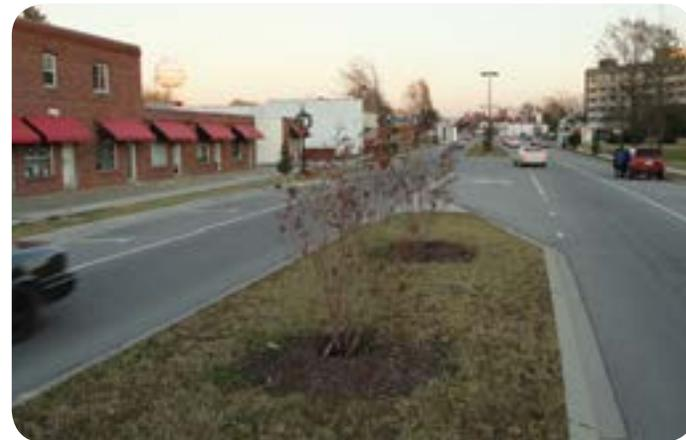
**Curb radius reductions:** A wide curb radius enables high-speed turning movements by motorists which can result in increased crashes with pedestrians and more serious outcomes when crashes occur. Reconstructing the turning radius to a tighter turn will reduce turning speeds, shorten the crossing distance for pedestrians, and also improve sight distance between pedestrians and motorists.
