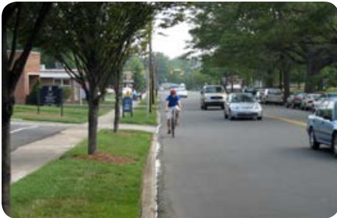
**Bicycle Boulevards:** Bicycle boulevards are streets with low motorized traffic volumes and speeds, designated and designed to give bicycle travel priority. Bicycle Boulevards use signs, pavement markings and speed and volume management measures to discourage through trips by motor vehicles and create safe, convenient bicycle crossings of busy arterial streets. (NACTO)
