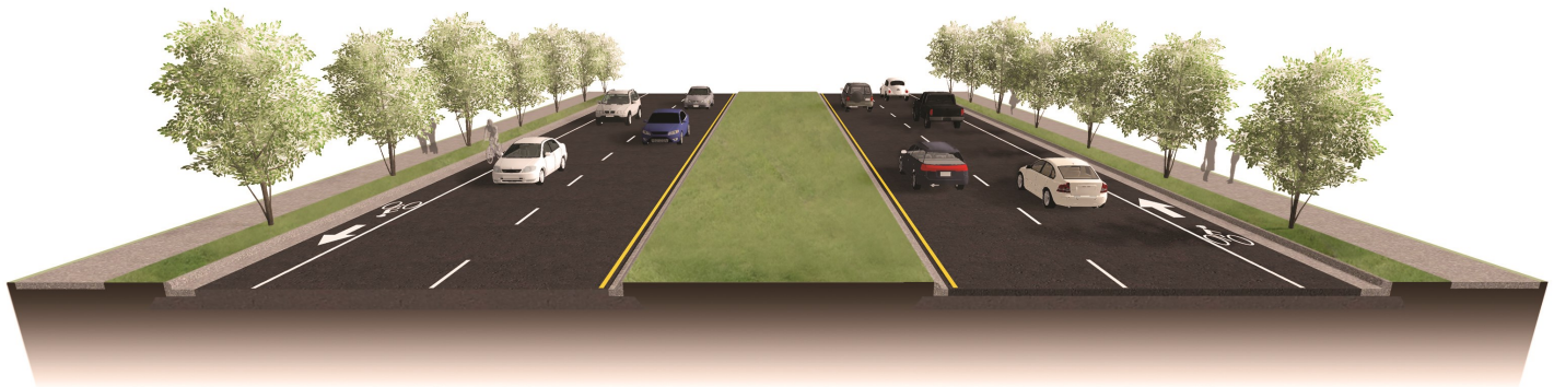
TYPICAL SECTION: FOUR LANES WITH MEDIAN, CURB AND GUTTER, SIDEWALK ON ONE SIDE, A MULTI-USE PATH ON THE OTHER SIDE, AND BICYCLE LANES
