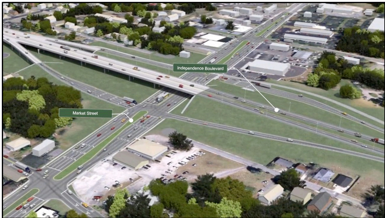
Figure 2-5: Tight Urban Diamond Interchange
