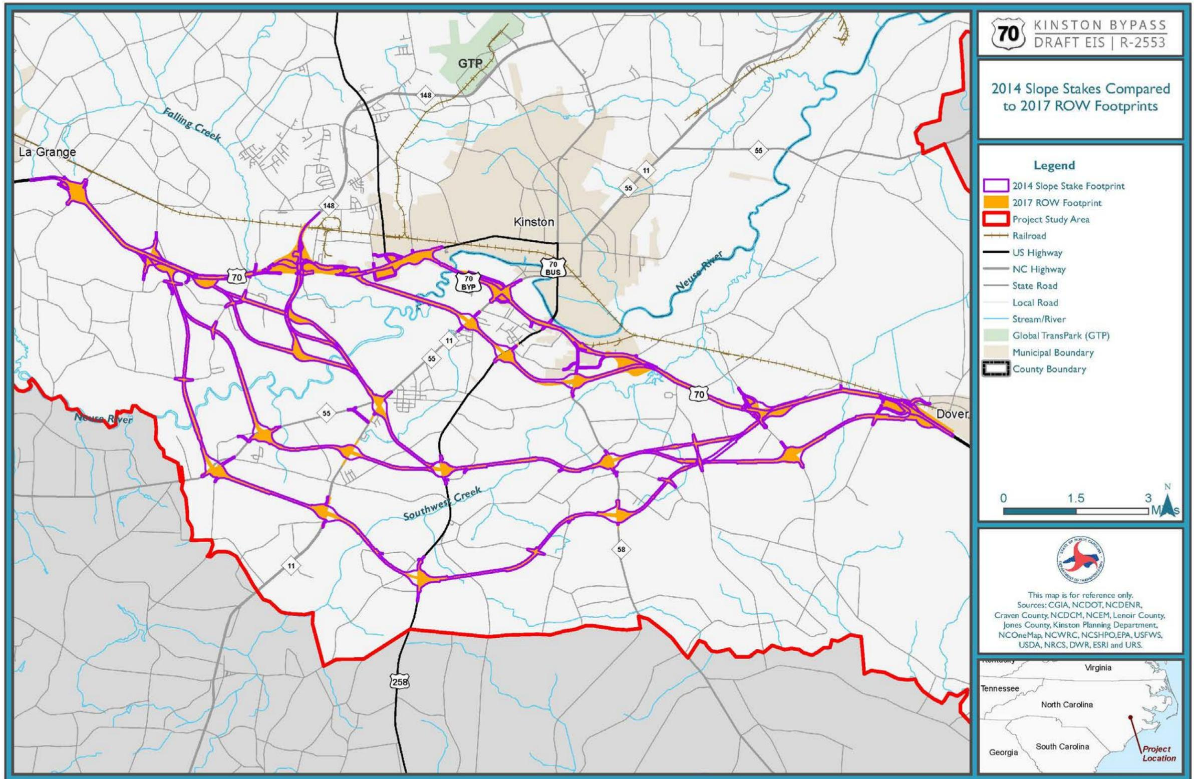
Figure 25. Comparison of 2014 Design and 2017 Right of Way for Kinston Bypass
