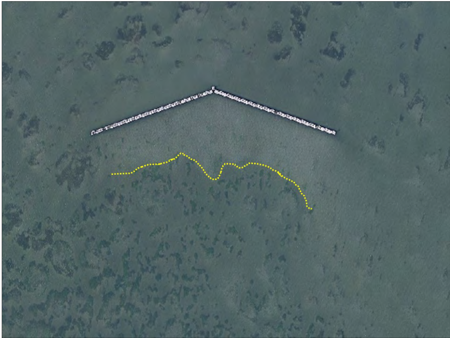
Figure 3. Sand apron south of wall visually outlined. 18 April 2018.
