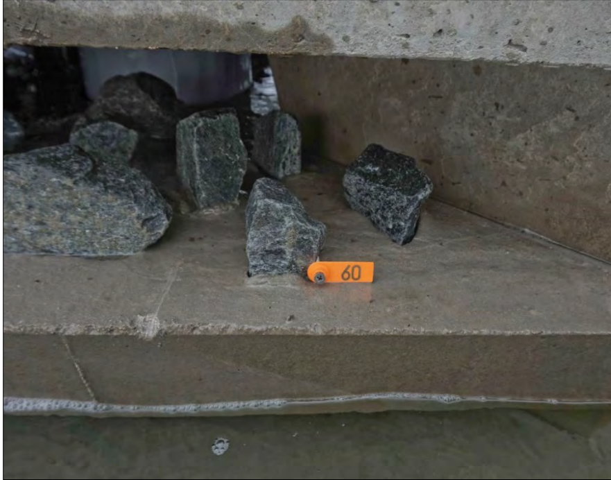
Photo 6. Example of numbered tag installed at every monitoring station on the wavebreak at the Bonner Bridge Seagrass Mitigation Site.
