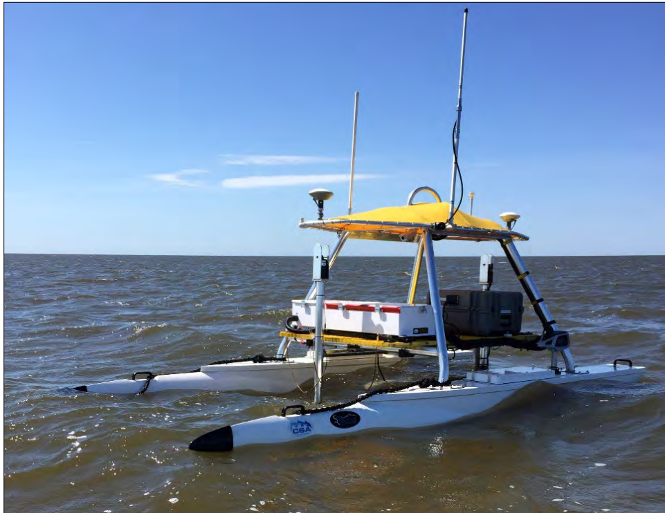
Photo 3. Unmanned surface vehicle (USV) collecting bathymetry data across the Bonner Bridge Seagrass Mitigation Site.
