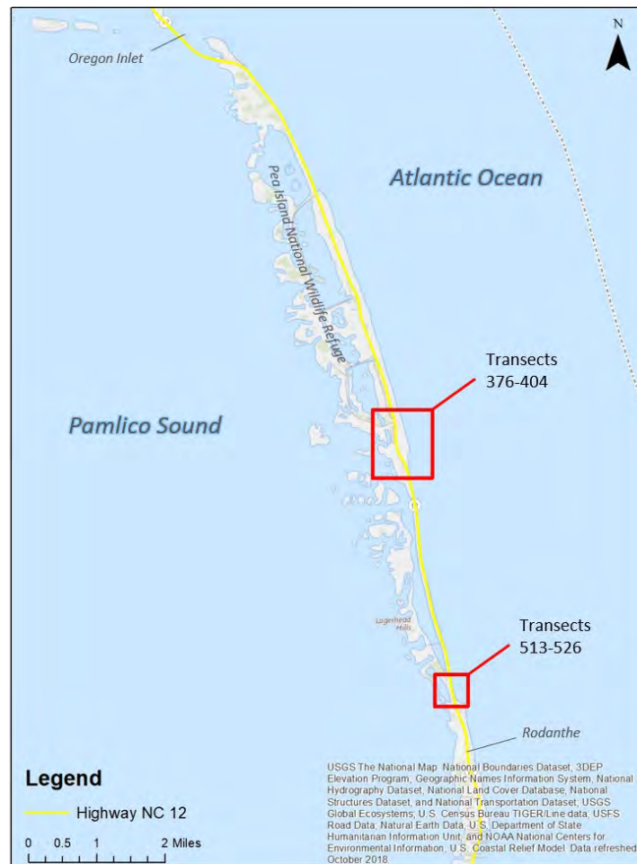
Figure 1 The regions outlined in red were altered due to changes in the edge of pavement (EOP) of Highway NC 12. These locations are near the Interim Bridge and the staging area for the new Jug Handle Bridge.
