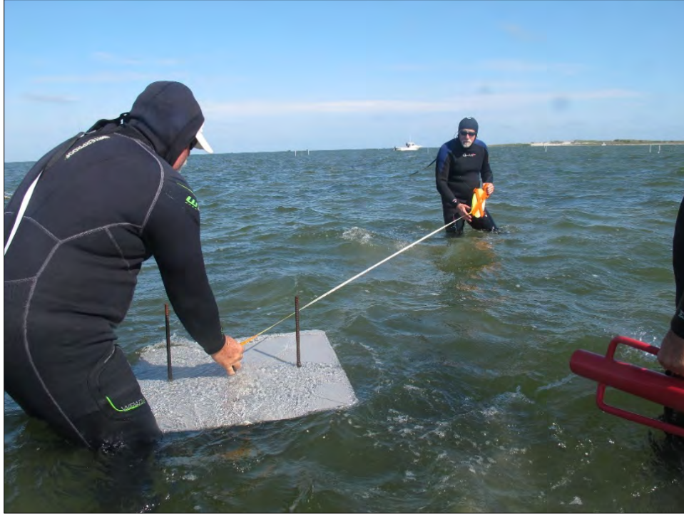
Photo II-2. Scientists measuring from the center rod to the edge of the seagrass patch on the randomly selected direction at the Bonner Bridge Seagrass Mitigation Site.
