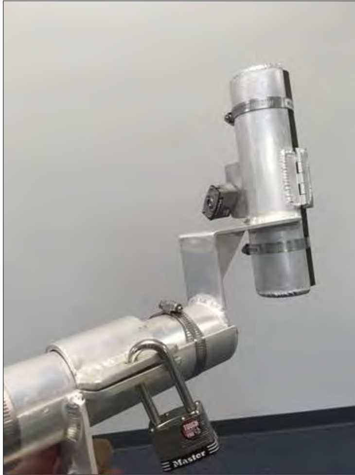
Photo 5. Re-engineered wave sensor bracket installed in January 2018 to hold the sensor vertical and further away from the sand surface.
