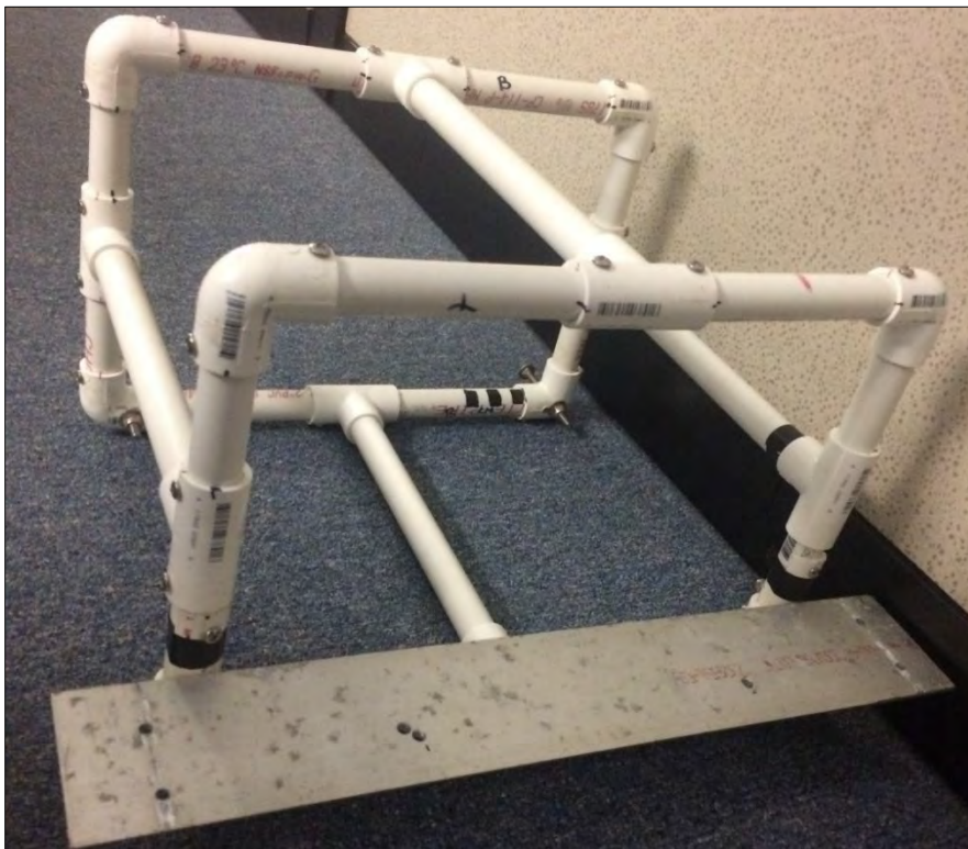
Photo 7. PVC camera mount framer used to photograph every monitoring station on the wavebreak at the Bonner Bridge Seagrass Mitigation Site.
