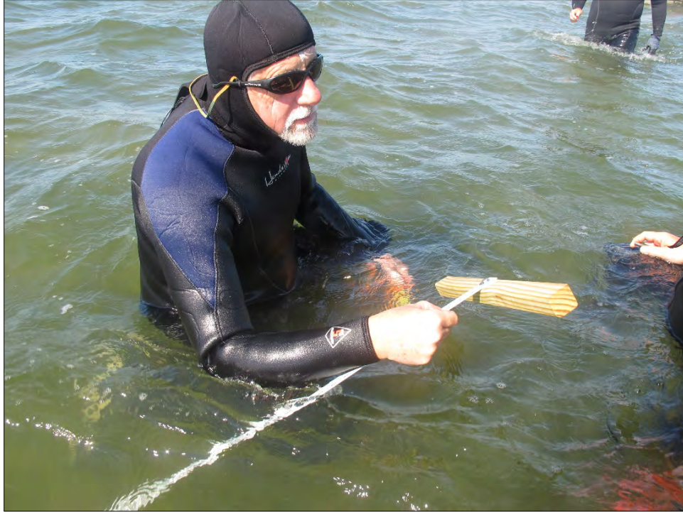
Photo 2. Inverted “T” shape ruler used to measure rod height above or below the substrate at the Bonner Bridge Seagrass Mitigation Site.
