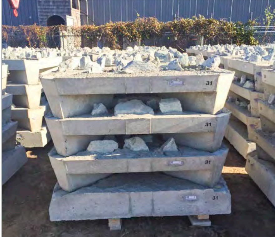
Photo I-2. One Reefmaker unit consisting of one base unit on the bottom and three wave attenuator units containing granite rock. One hundred and one of these units were installed at the Bonner Bridge Seagrass Mitigation Site. For scale, the width of the units is 4.8 ft (1.46 m).
