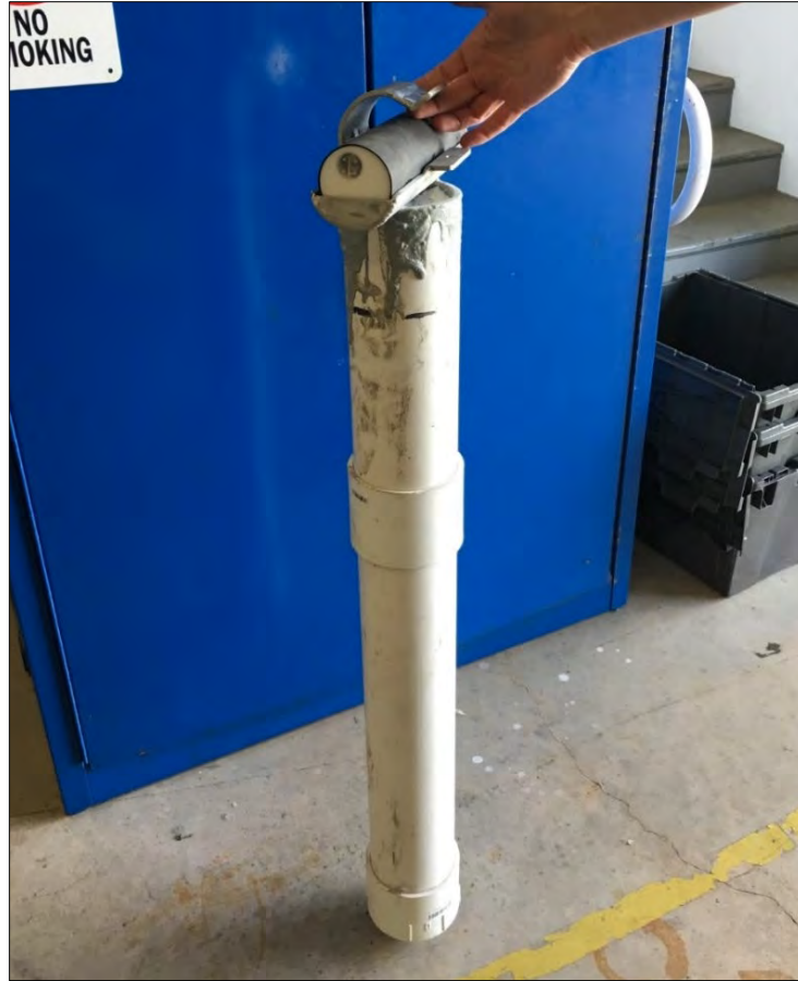
Photo 4. Photograph of one of the two wave sensor brackets cemented into its base, prior to installation at the Bonner Bridge Seagrass Mitigation Site. The hinged bracket is shown being lifted; a disposable padlock is installed through the hinged piece to keep the sensor secure.
