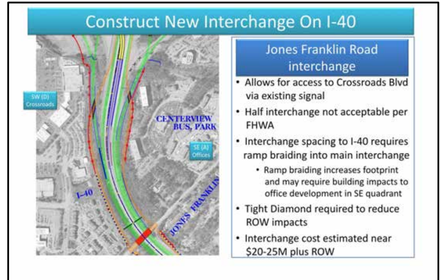
Figure D-8. Construct New Interchange on I-40 – Option 3
