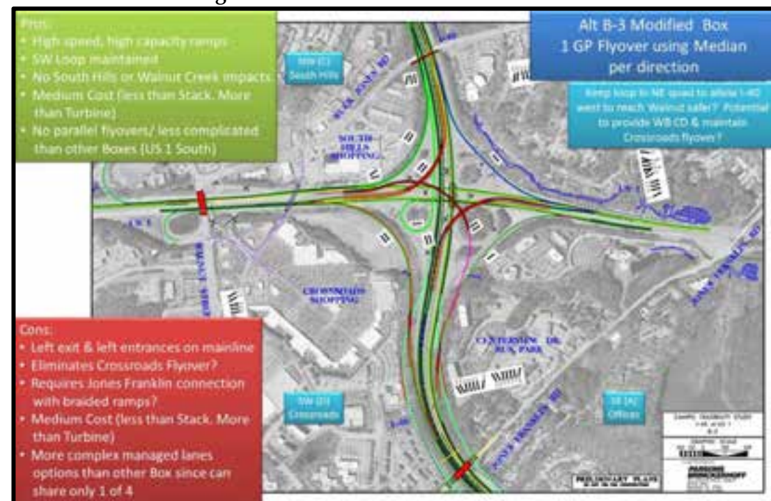
Figure D-15. Alternative B-3 Modified Box
