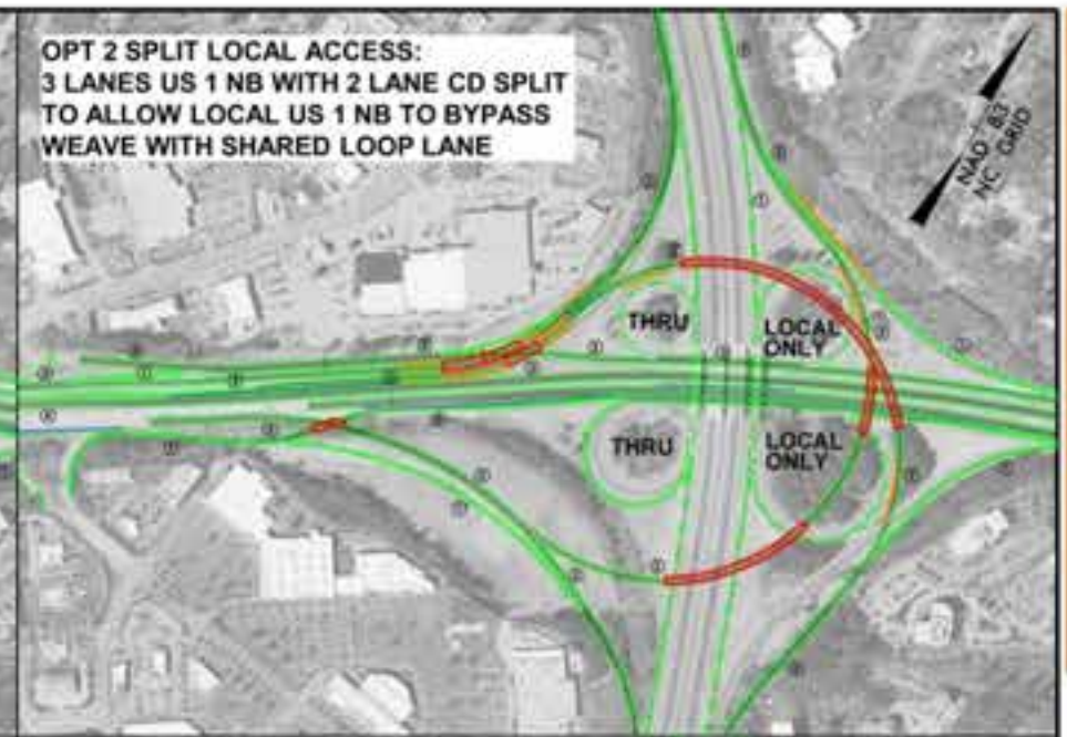
Figure D-12. Options for Connecting US 1 NB CD
