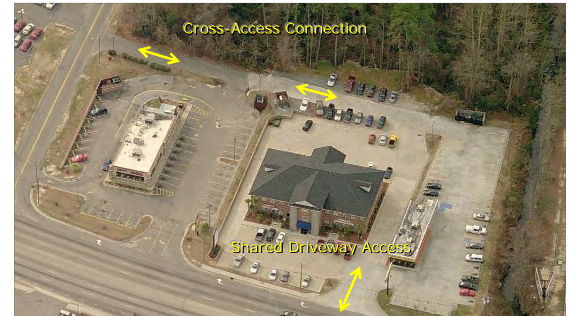
Shared Driveway Access and Cross-Access Connection
