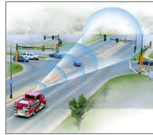
Emergency Vehicle Preemption
